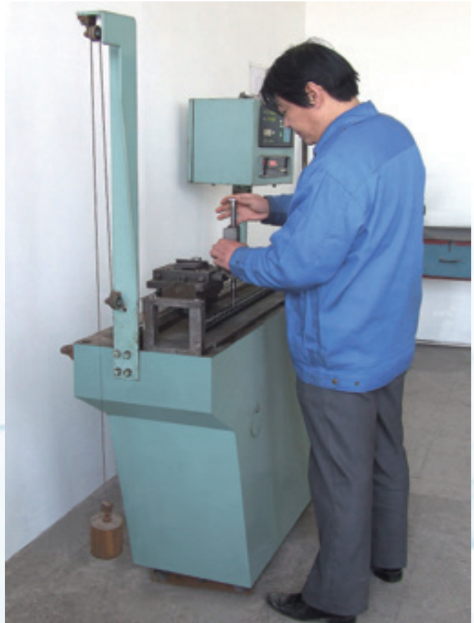
链长精度测试 Accuracy Test of Chain Length
